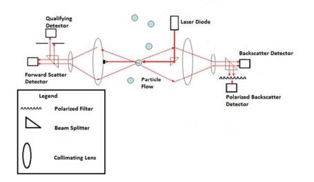
Figure 1A. A schematic of the CASPOL instrument adapted from DMT Manual (2011).
